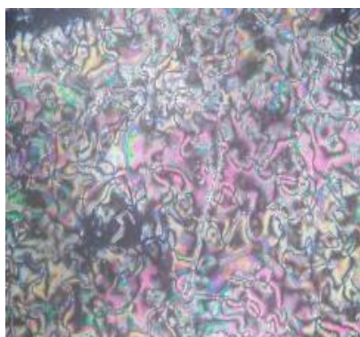
Threaded marble texture of compound P-Decyloxybenzylidene P-Toluidine @ 74.9 ° C
