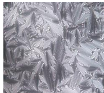
Arced focal conic fan texture of compound P-Decyloxybenzylidene P-Toluidine @ 63.5 ° C
