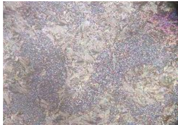
Sanded texture of Smectic A Phase @ 96.7 ° C of the compound P-Cyanobenzylidene P-Nonyloxyaniline
