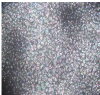
Nematic droplet texture of compound P-Decyloxybenzylidene P-Toluidine @ 76 ° C
